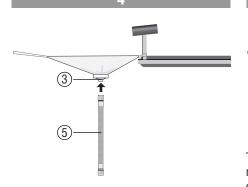
The (separately available) corrugated tube (5) can now be pushed onto the discharge nozzle (3) of the Apron.
