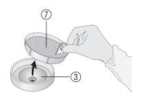
The filter sieve (7) holds back tissue fragments and thus prevents the conduit from becoming blocked. It can be removed from the discharge nozzle (3).
